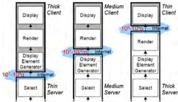
Fig. 2. Thick, medium, and thin 3D client architectures with orders of magnitude of geometries (g) and image data (p).
